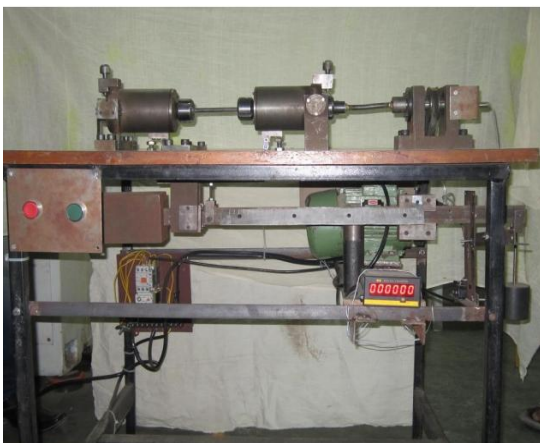
Photograph 9- Fatigue test set up
