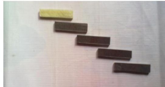
Photograph 5- Impact test specimen
