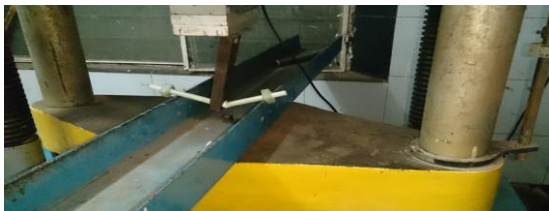
Photograph 4- Composite specimen after flexural load
