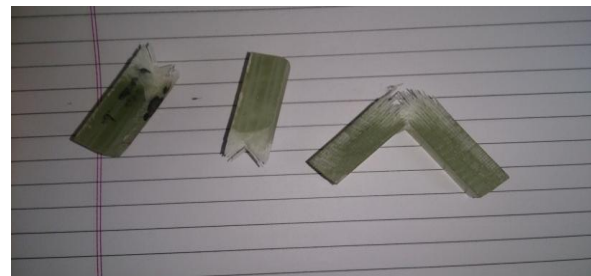
Photograph 7- Composite specimen after test
