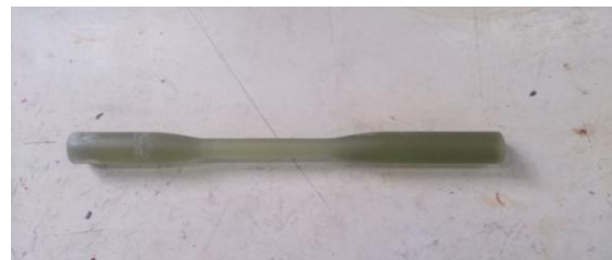
Photograph 2- Composite specimen for Tensile test
