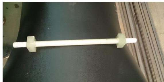
Photograph 1- Composite axle made by pultrusion process
