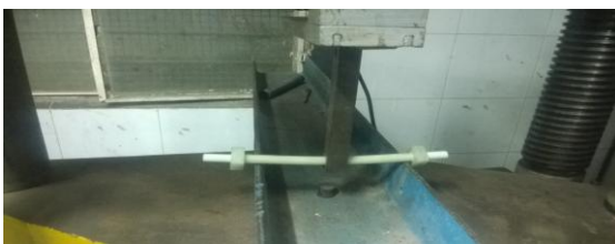
Photograph 3- Three point bending test set up
