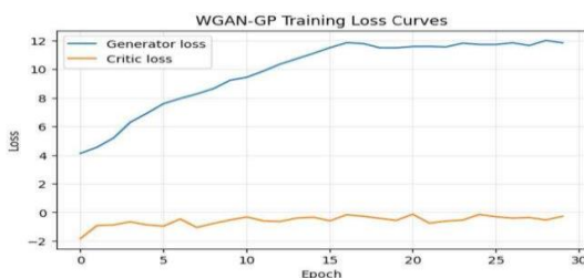
Figure 4.2. WGAN-GP training loss curves for v2 (10-dimensional spectral and morphological feature set). The generator loss reaches a higher plateau of approximately 11.5–12.0, reflecting the greater complexity of the augmented feature space. The critic loss follows the same convergence pattern as v1.
