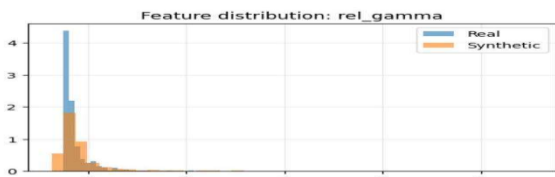
Figure 4.15. Marginal distribution histograms for rel_gamma (v1, best test recording). The most extreme marginal mismatch of any feature: the real distribution is an exceptionally narrow spike (peak density \sim 4.4 ) while the synthetic distribution is broadly spread across approximately ten standard deviations. This feature is the most probable primary driver of the observed KS max statistic for this recording.
