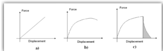
Fig.2- Different behaviours of the fastener joints a) linear Elastic behaviour, b) Non-linear Elasto-plastic behaviour, c) damage Behaviour
