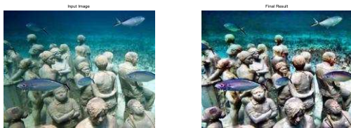
Fig. 10 First image is the input image and second image is the final result with Gain constant = 5; p = 11
