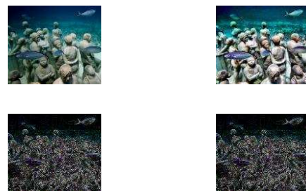
Fig.7 Top line images are the first and second input; bottom line images are the Local Contrast Weight applied to each input
