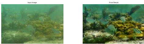
Fig. 9 First image is the input image and second image is the final result with Gain constant = 150; p = 10
