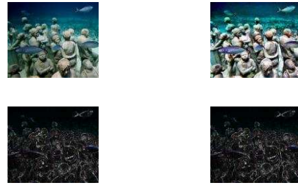
Fig.5 Top line images are the first and second input; bottom line images are the Laplacian Weight applied to each input
