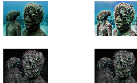
Fig.6 Top line images are the first and second input; bottom line images are the Laplacian Weight applied to each input
