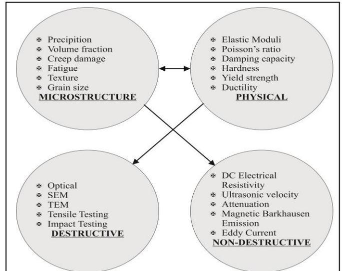
Figure 1. Correlation between microstructure, physical and mechanical properties of the material
