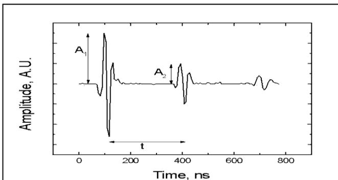
Figure 6. RF signal showing first and second back wall echo. ( $A_1$  and  $A_2$ )
