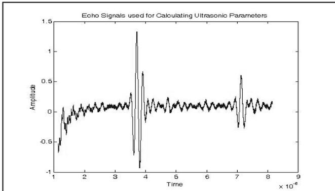
Figure 5. RF signal of Solution Annealed IN-718 specimen
