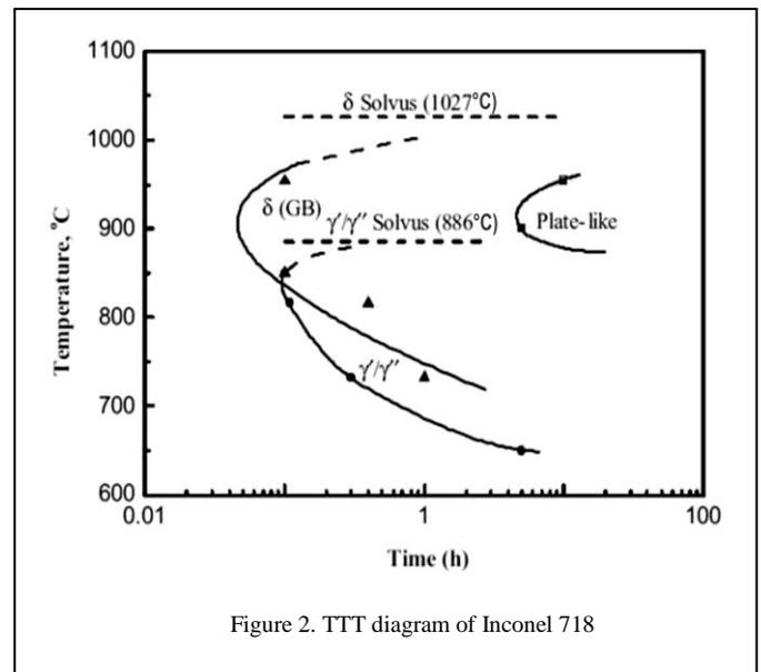
Figure 2. TTT diagram of Inconel 718
