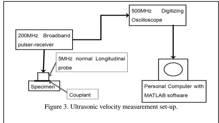
Figure 3. Ultrasonic velocity measurement set-up.
