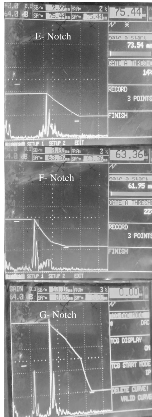
Fig. 8: DAC curve for E, F, G notches on maraging steel plate for reference 64 dB
