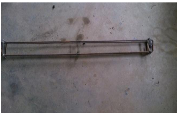
Fig.5. Reinforcement cage for shear behaviour
