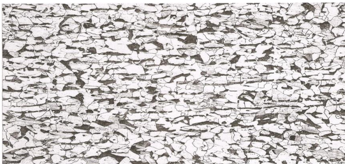
Fig 1.8 Grain Structure of Ferric Parent Steel Material
