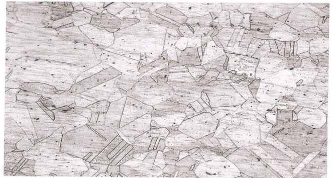
Fig 1.11 Grain Structure of Welded Stainless Steel Material
