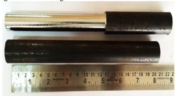
Fig.1.4 Mild steel rod and turning has been done up to 12.5 cm
