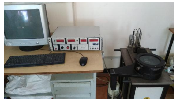
Fig. 3. Pin-on-disc wear test setup
