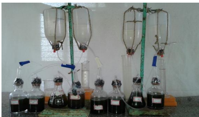
Fig 5: Biogas production setup
