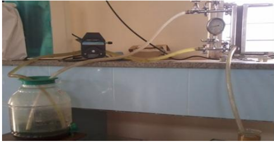
Fig 3: Cross flow filtration
