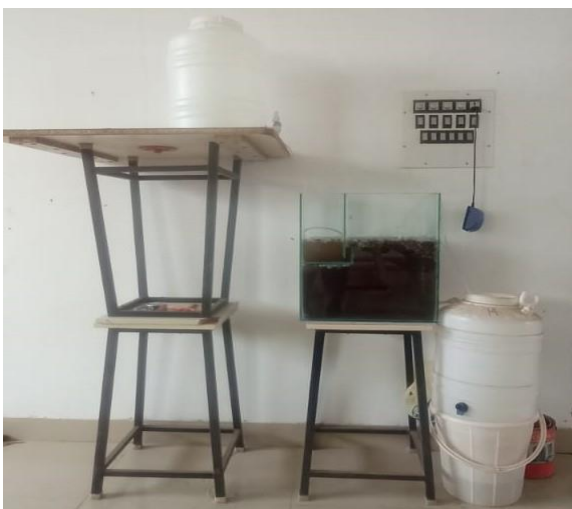
Fig.2 experimental setup of lab scale MBBR system
