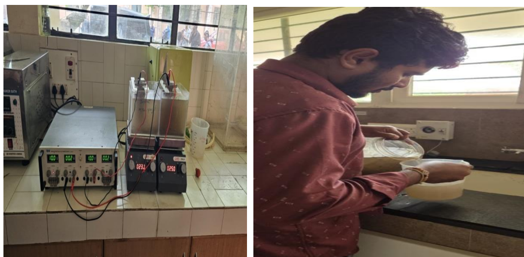
Fig 1: Experimental set up for treating automobile wastewater and collection of wastewater
