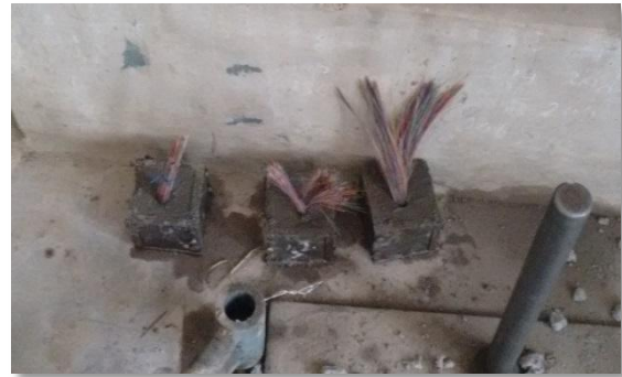
Figure 1: Translucent Concrete Cubes
