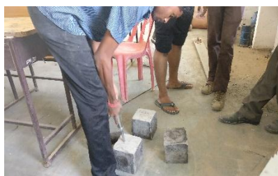
Fig 5: Rebound Hammer Test
