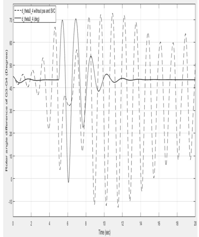
Fig. 8. Rotor angle difference of G3 to G4.
