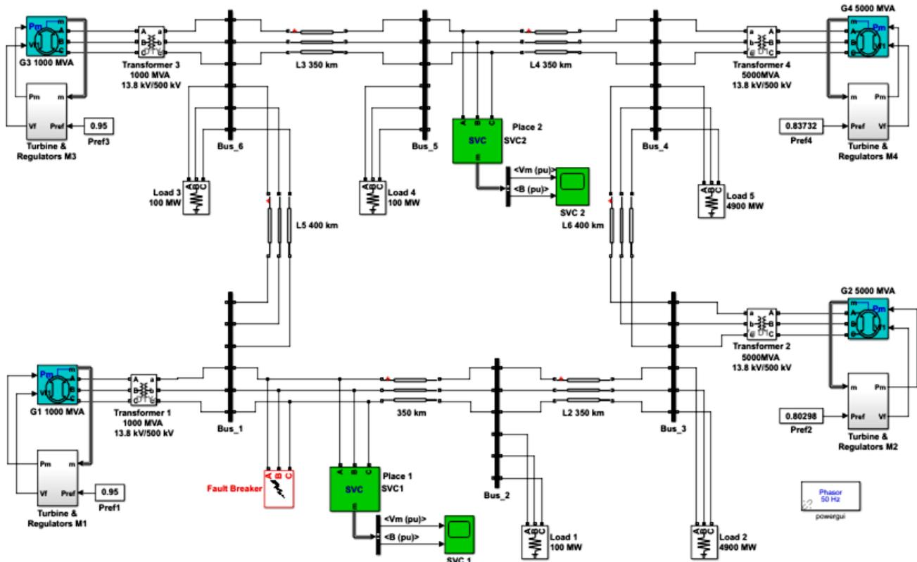
Fig.6. Test system (4 machine, 6 bus) modeled in Simulink/MATLAB.
