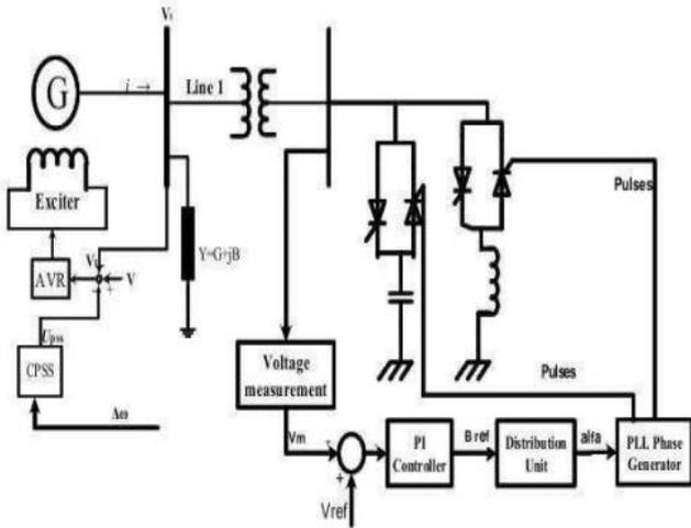
Fig.3. single-line diagram of a SVC and a simplified block diagram of its control system.
