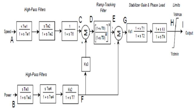
Fig.2. Accelerating Power PSS Model.
