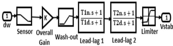
Fig.1. Block diagram of the PSS.
