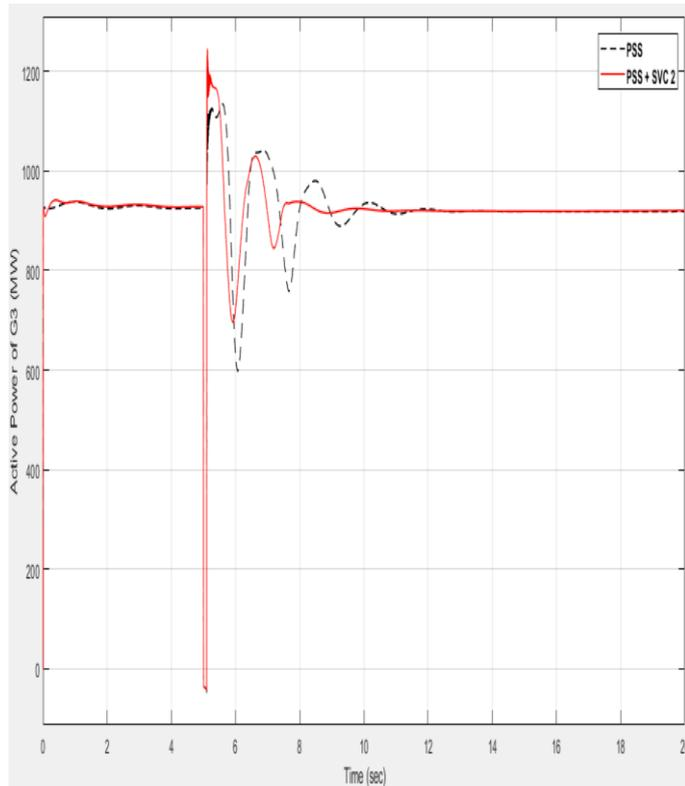
Fig. 22. Transmission line active power of G3.
