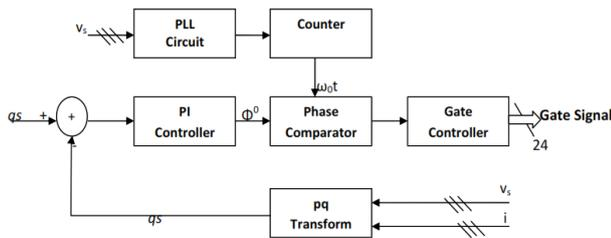
Fig.5. Block Diagram of SVC Control Circuit.
