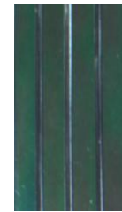
Figure 7: Heated ribbed plate with LC on surface
