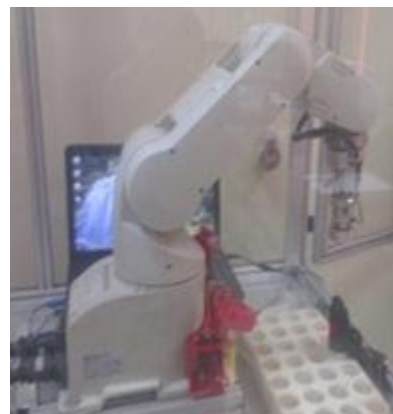
Fig. 3. Experimental setup (Mitsubishi® RV-2AJ) educational manipulator
