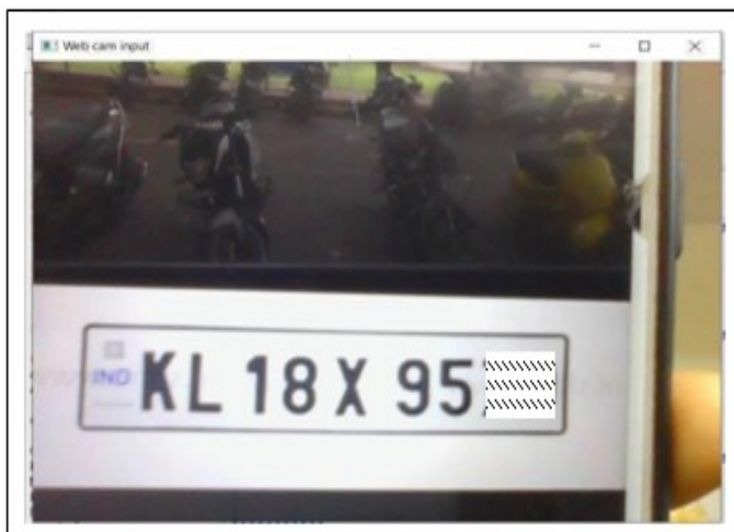
Fig.2. license plate is captured when helmet is not detected
