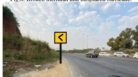
Fig.7. There is no warning sign provided on the curve.
