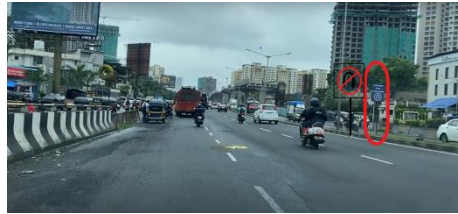
Fig.9. The regulatory sign is confusing as there is no U-turn on the flyover.
