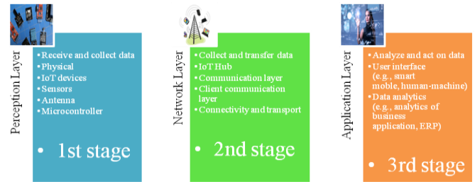
Fig.4. General IoT Systems Architecture
