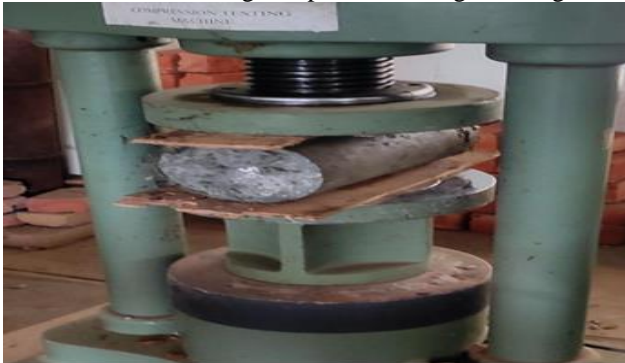
Fig 3.3 Tension testing on compression testing machine
