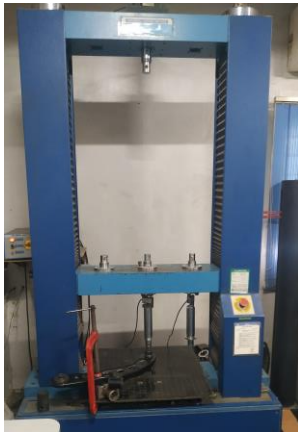
Fig. 15 Testing of LCA under UTM
