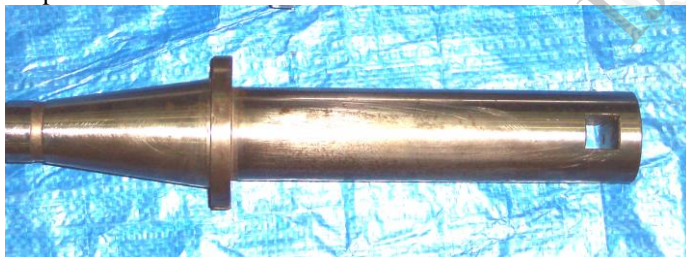
FIG.3.4: Boring bar showing placement of the tool
