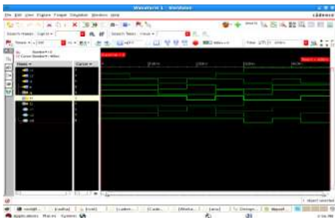
Fig 16 Output waveform Negative enable D latch
