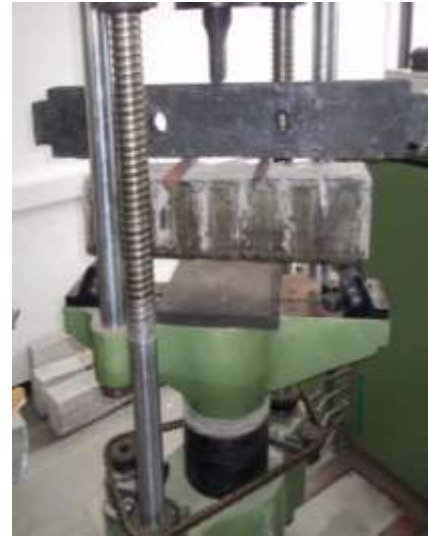
Fig.3.1 Testing of UVS Beam
