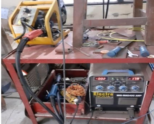
Fig.1. MIG Welding setup
