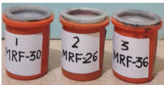
Figure 2: Prepared three Samples of MR Fluid with different volume Fraction
