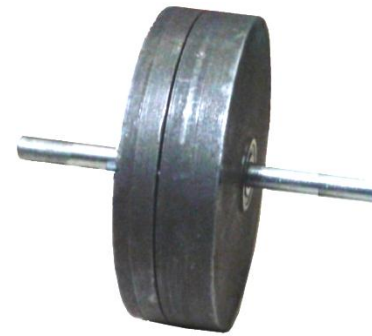
Figure 5. MR fluid Brake
