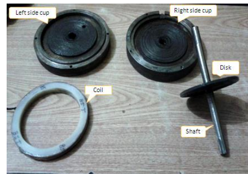
Figure 6. Different components of MR fluid Brake
