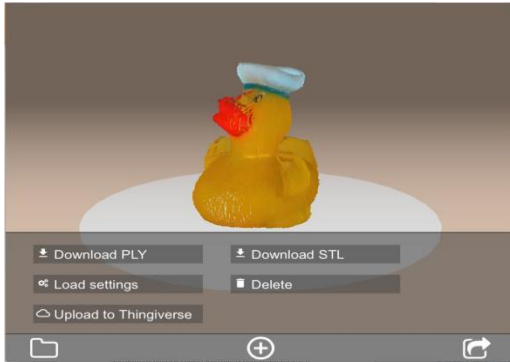
Fig. 5 Sharing dialog. Offers the opportunity to download scans in different formats and delete scans.
