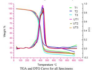
The degradation temperatures at different level of Thermogravimetric weight loss for the composites.
