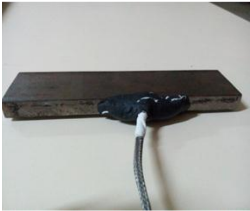
Fig. 4 Workpiece with embedded thermocouple
