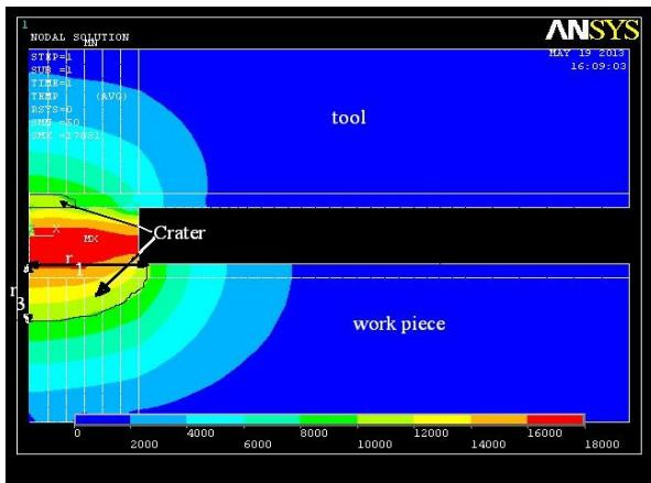
Figure 8 Temperature distribution obtained for a Current intensity value of 68 amps
