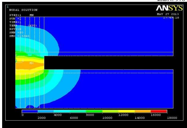
Figure 9: Temperature distribution obtained for a current intensity value of 58 amps
