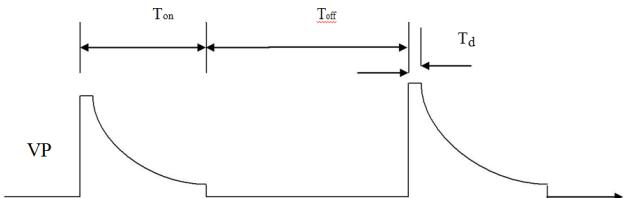
Figure 6: Series of electrical pulses at the inter electrode gap
