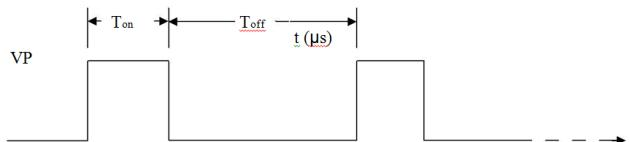
Figure 5: Graphical representation of sparking cycles
