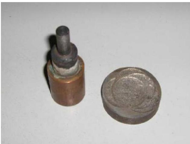
Figure 7: Electrode and work piece after the machining operation.
