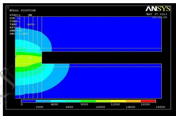
Figure 10: Temperature distribution obtained for a current intensity value of 44 amps
