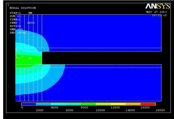
Figure 11 Temperature distribution obtained for a Current intensity value of 36 amps
