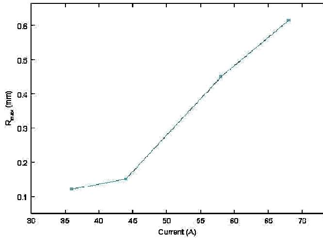
Figure 13: Rmax values with various current intensities for FEA
