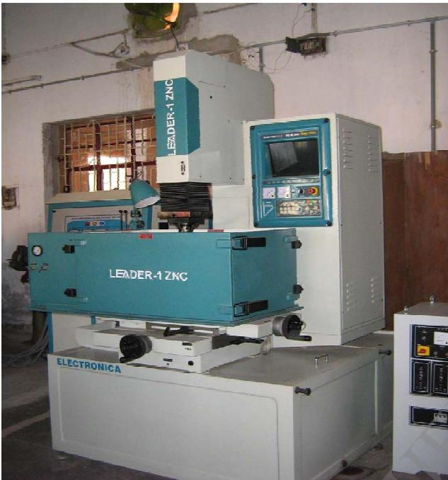
Figure 3: EDM machine used for the experiment
