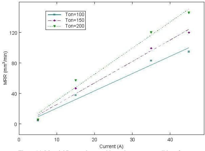
Figure 14: Material Removal rates with varying current conditions for Experiment.
