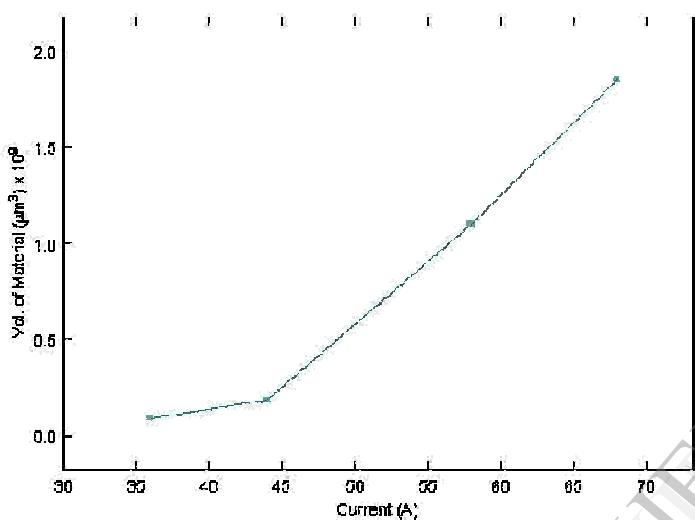
Figure 12: Volume of material removed with different current intensities for FEA
