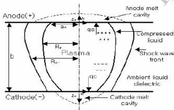
Figure 1: Plasma channel developed during on-time
