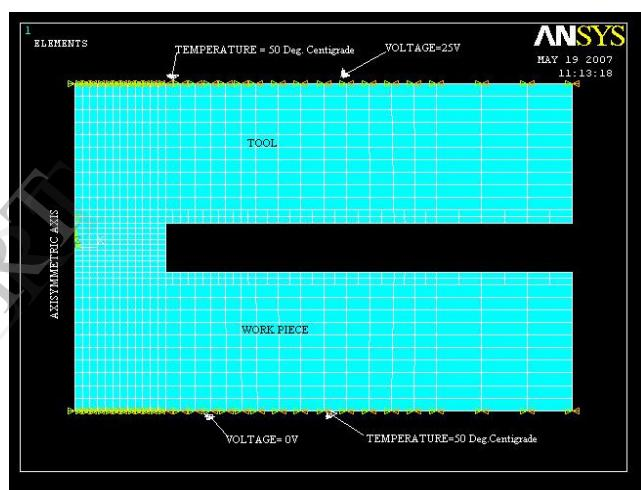
Figure 2: Elements after meshing and application of loads
