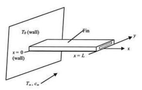
Here we take a longitudinal slot on the fin in order to increase the surface area of the system. Now taking the same parameters as considered earlier, the heat transfer rate at various lengths can be calculated as follows.
