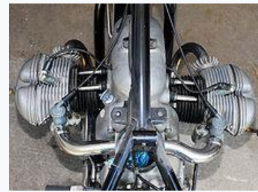
Fig-1.4. Air-cooled boxer engine on a 1954 BMW motorcycle
