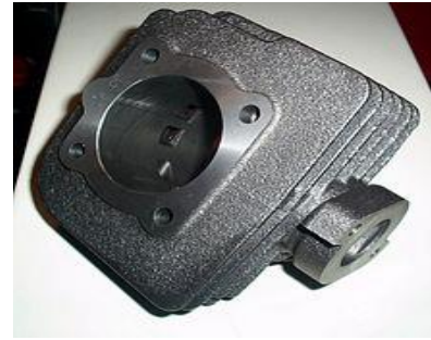
Fig-1.3. Malossi air-cooled cylinder for two-stroke scooters. The exhaust port is visible to the right.
