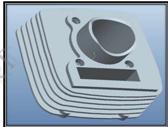
Fig.3. Pro/E model of Rectangular fin (2.5 mm thickness)
