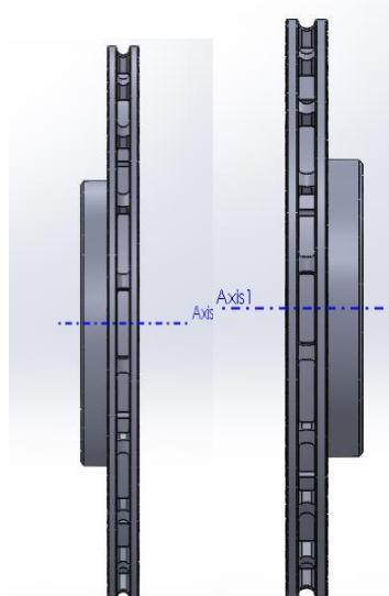
The models of the rotors are modeled on SOLIDWORKS 2020 SP0 and is imported for transient state analysis on ANSYS 2021 R1. This analysis is done in the time duration of 13 seconds, which is the time required for the vehicle to come to rest from 200Kmph.
