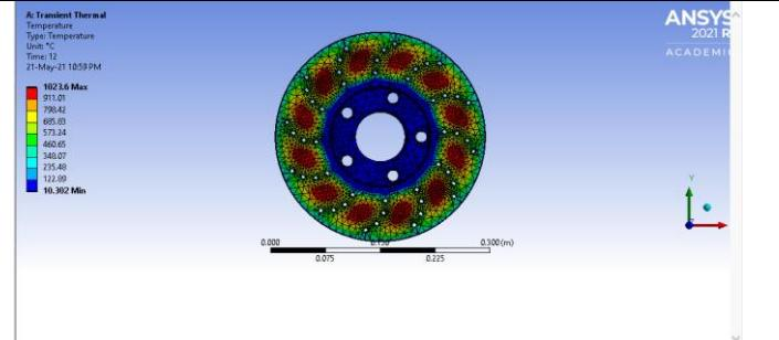
The End result of analysis on Gray Cast Iron Rotor disc.
