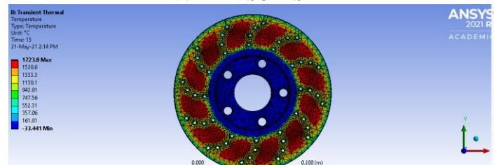
The end result of the analysis on Stainless Steel rotor disc.
