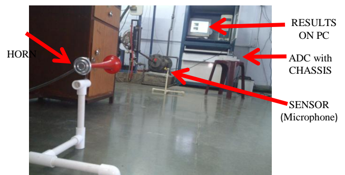
Fig. 14. Actual setup for data acquisition of sound pressure
