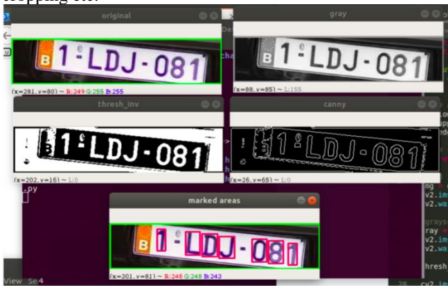
Fig.7: Segmentation by converting to grayscale
