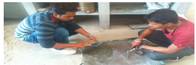
Fig.3:- Mixing &amp; filling of cement paste in mould
