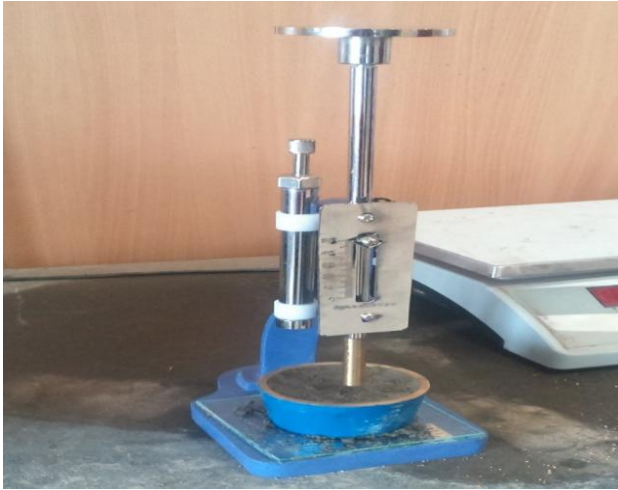
Fig.5:- consistency test of cement
