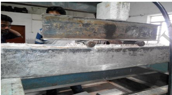
Fig 5(b) Crack pattern for retrofitted beam
