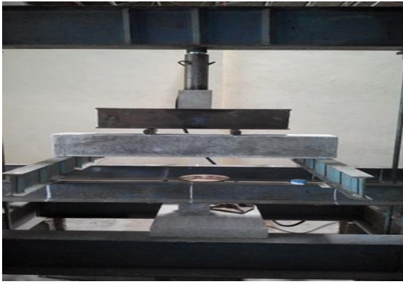
Figure 4 Test set up (Loading Frame)
