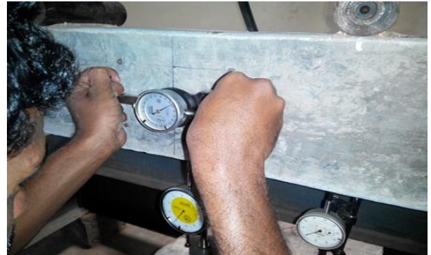
Fig 15 measuring strain with demec gauge
