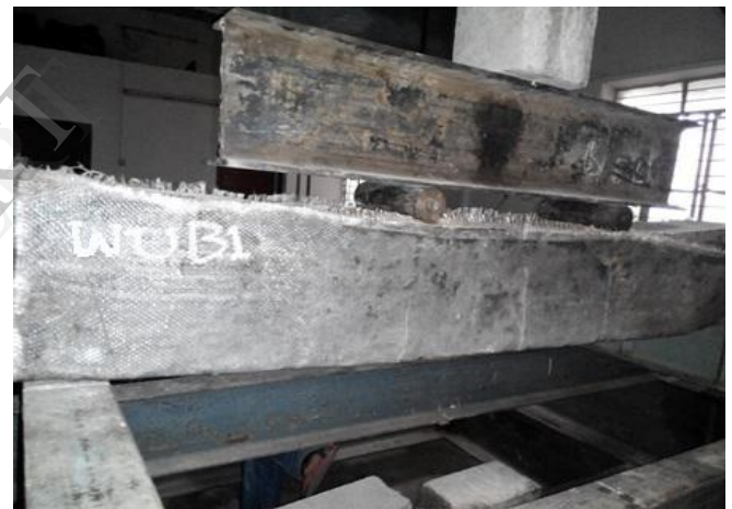
Fig 12 A typical failure pattern of retrofitted RC beam
