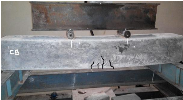
Fig 5(a) Crack pattern for control beam
