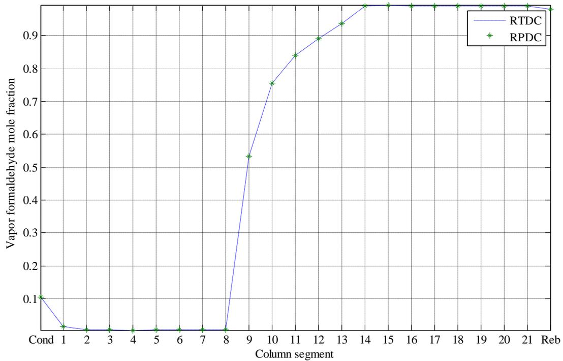
Figure 9. Vapor formaldehyde mole fraction profiles of reactive tray and packed distillation columns
