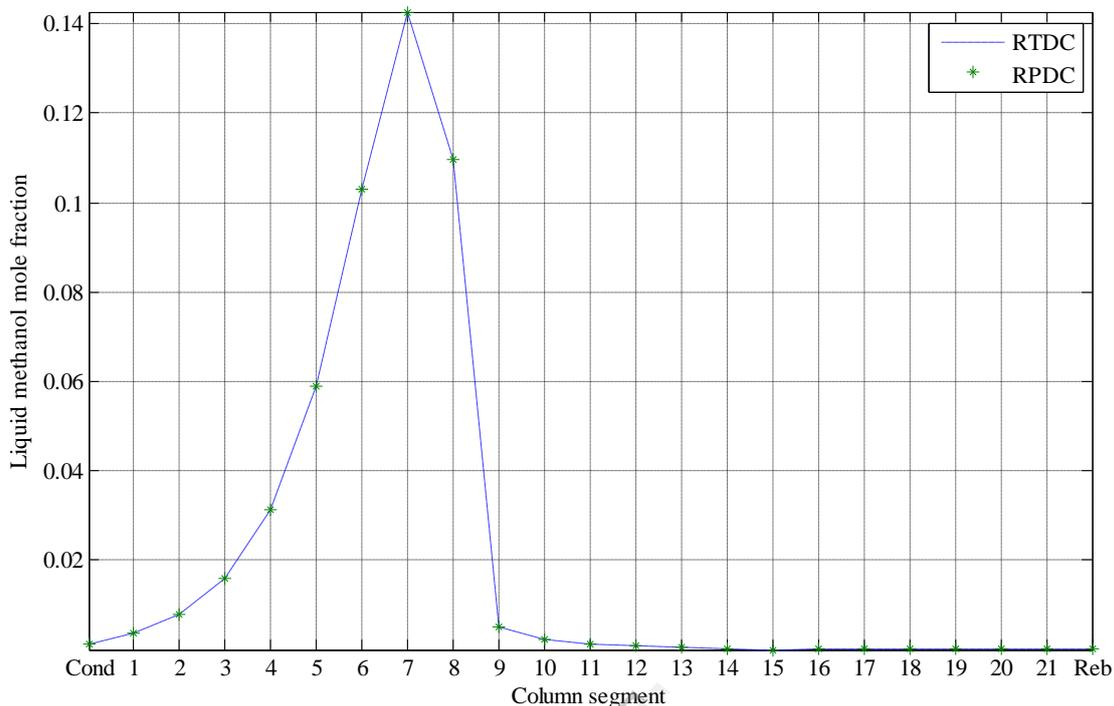
Figure 4. Liquid methanol mole fraction profiles of reactive tray and packed distillation columns
