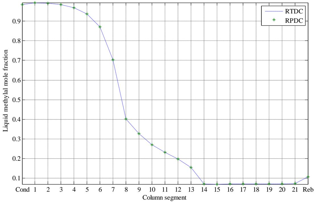
Figure 6. Liquid methylal mole fraction profiles of reactive tray and packed distillation columns
