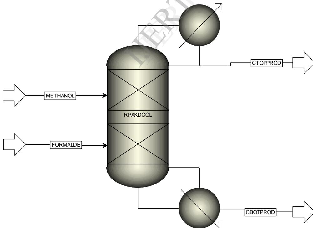
Figure 2. Reactive packed distillation column for the production of methylal
