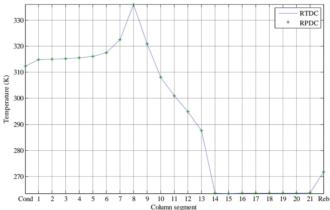
Figure 3. Temperature profiles of reactive tray and packed distillation columns
