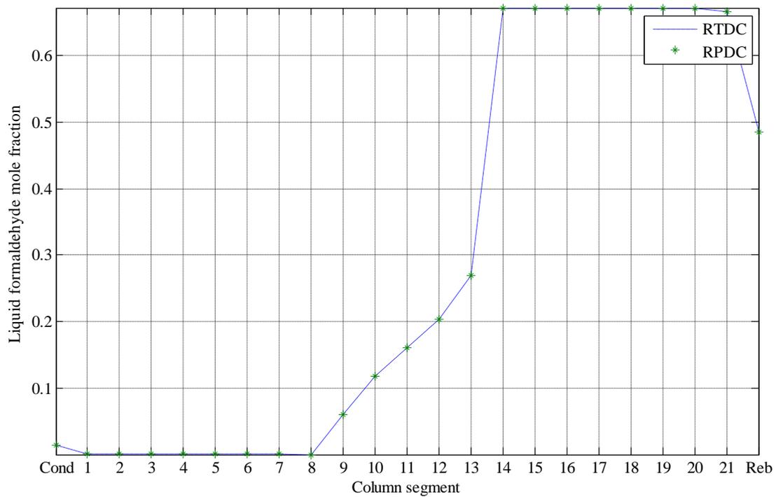
Figure 5. Liquid formaldehyde mole fraction profiles of reactive tray and packed distillation columns
