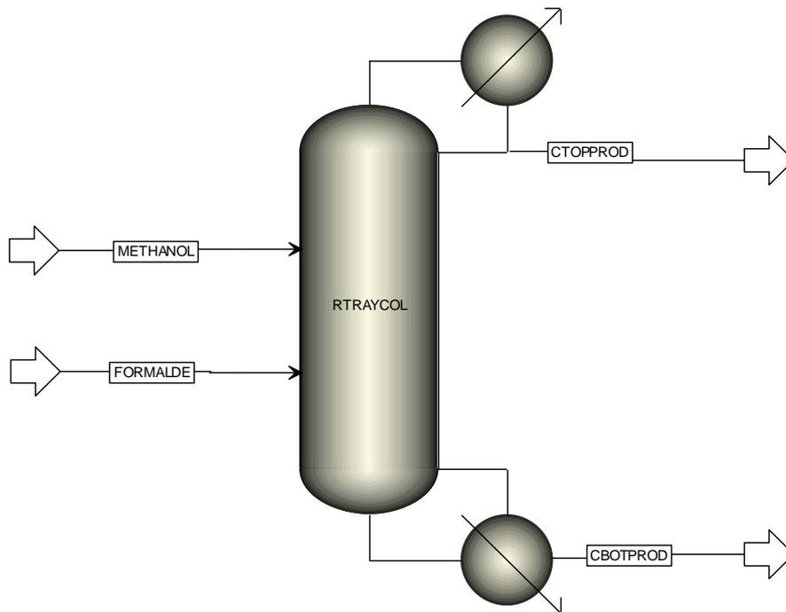
Figure 1. Reactive tray distillation column for the production of methylal
