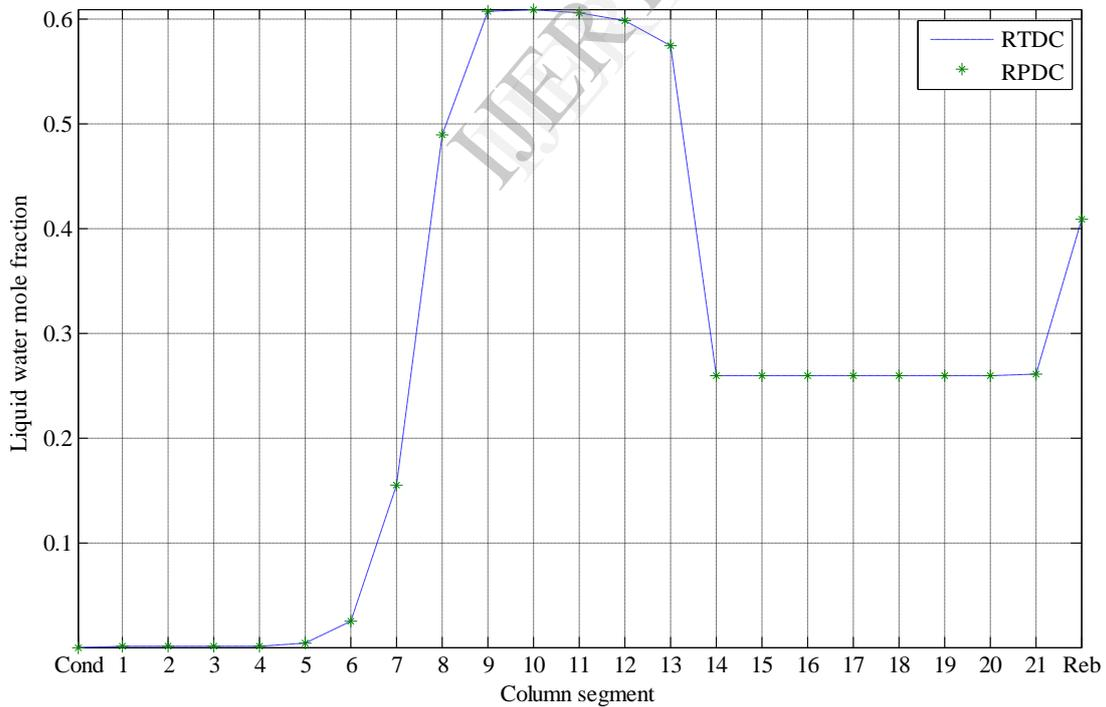
Figure 7. Liquid water mole fraction profiles of reactive tray and packed distillation columns
