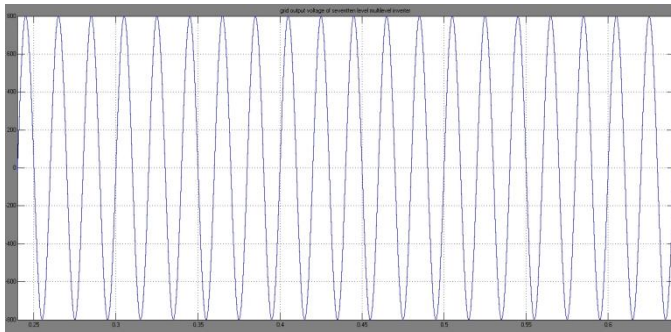
Fig.28 shows the asymmetrical cascaded H-bridge seventeen level multilevel inverter with grid connected of pure sine wave output voltage
