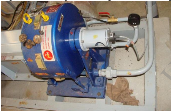
Fig.2.5. Eddy current dynamometer for loading
