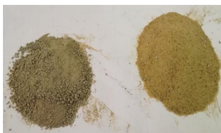
Figure1: GGBFS compared to sand sample
