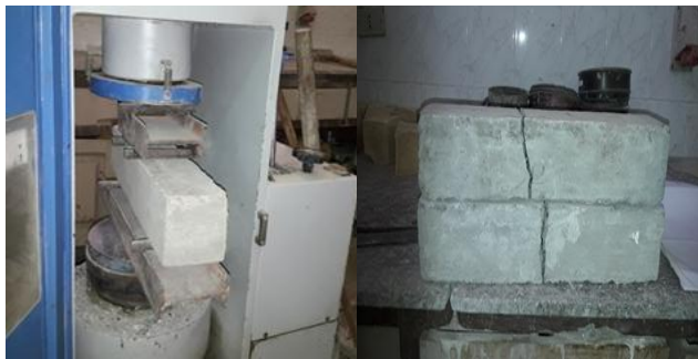
Figure. 3: Compressive and flexural tests
