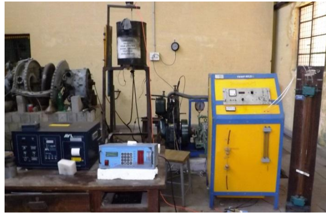
Fig 2. Experimental setup of LHR Engine Test rig
