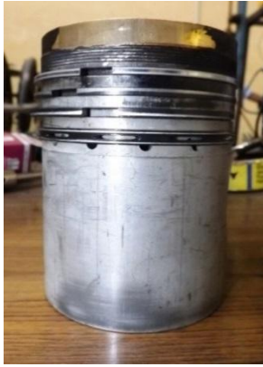
Fig. 1 Photo Graphic View of Aluminium Piston with Brass Crown and Air Insulation
