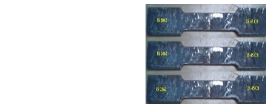
Fig 5: Specimen sampling from the weld pads
