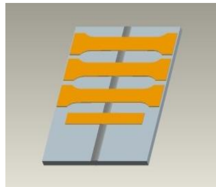
Fig 5: Specimen sampling from the weld pads
