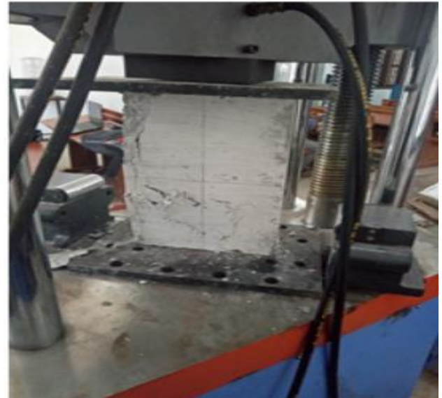
Fig 5: Failure and crack pattern of short columns
