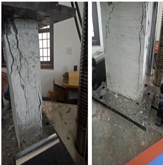
Fig 4: Failure and crack pattern of short columns
