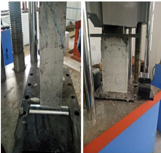
Fig 3: Failure and crack pattern of short columns
