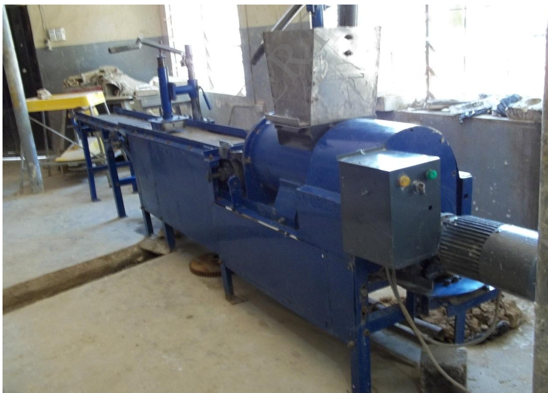
Fig. 12: The Developed Tile Making Machine Source: Morakinyo (2012)
