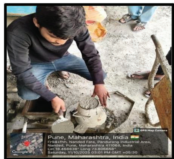
Figure 5 Slump Cone Test on Fresh Concrete
