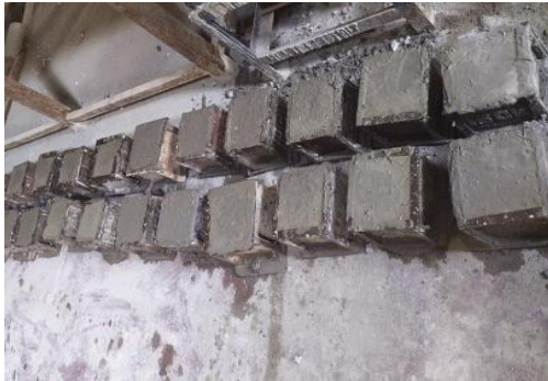
Fig 6. Sample of cube casting
